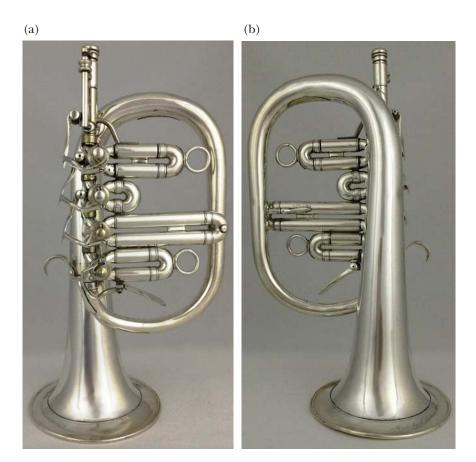
Figure 6. Cornet in E-flat, silver, with four Allen flat-windway valves, inscription along the bell rim: "Made by J. Lathrop Allen, No. 111 E. 18th St. N. Y." (a) left side; (b) right side. Photos courtesy of the J. Loyd Davis Collection, Prairie Village, Kansas.
