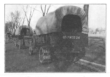
A REAR view of the truck column. Battery personnel, as well as ammunition, are carried in the trucks. The shoeplates, as illustrated, are readily attached to the rear wheels for travel over difficult terrain.
