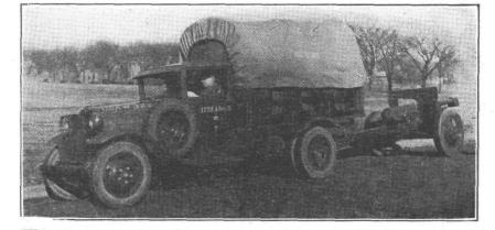
THE standard 1½ ton commercial truck, loaded with 100 rounds of ammunition and pulling the 75 mm. gun. The latter has the modified ball-bearing axle, disc wheels and pneumatic, puncture-proofed tyres. For firing, they provide a highly stable mount with minimum displacement.
