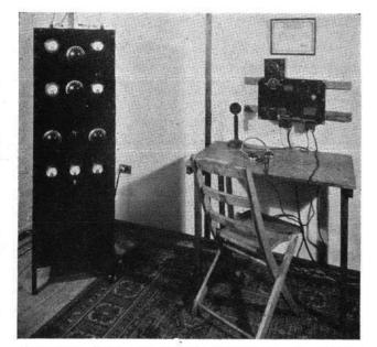
Transmitter (left) and Aircraft Transmitter and Receiver (right) of Station W8HJP
