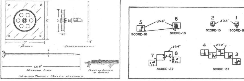
Fig. 6. Details of pulley.
